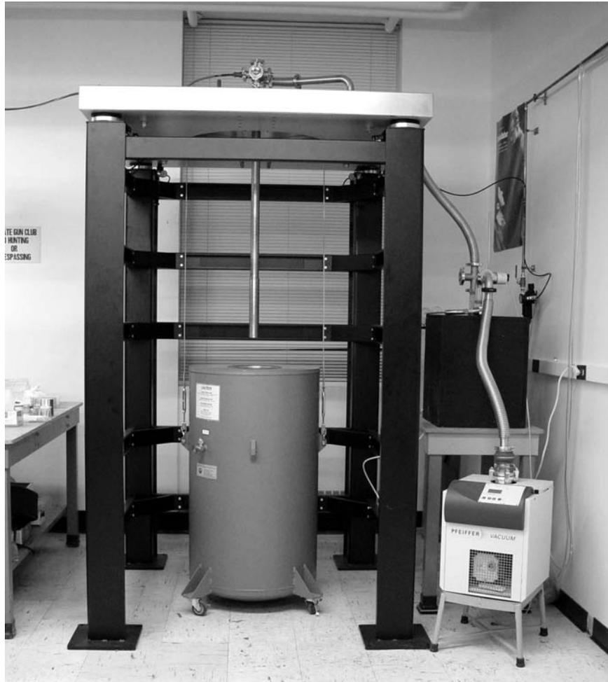
**Figure 3.4: Picture of the EFM including the probe, vibration isolation, and vacuum pump.**
