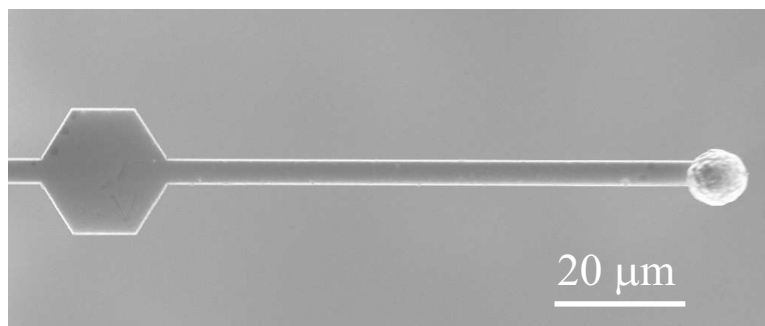
Figure 5.6: A scanning-electron micrograph of the end of the custom-fabricated cantilever and magnetic tip. The wider section of the cantilever is a laser reflection pad used for fiber-interferometric detection of the cantilever displacement. The tip is a 9 \mu\text{m} Ni sphere which was epoxied to the end of the cantilever.
